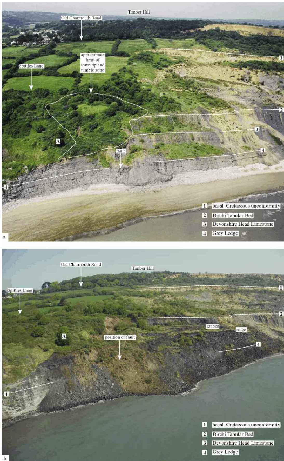
Figure 2. Before-and-after photographs of the May 2008 landslide. (a) Oblique air photograph of The Spittles and adjacent areas in July 2003, view north at about mid tide. West Dorset District Council (WDDC) Frame D01000001, copyright WDDC. (b) Approximately the same view taken on May 8th, two days after the landslide, at high tide. The red-brown material at the west end of the landslide is material from the town tip. Photographed by the Maritime and Coastguard Agency (MCA), copyright MCA. The approximate position of the boundary of the Lyme Regis Town Tip and the tumble zone are based on Anon (2007).
